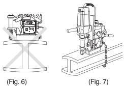
• 5 hours is the maximum continuous operating period for the Magnet. And 30 minutes is the rated operating period for the Drill Motor.
