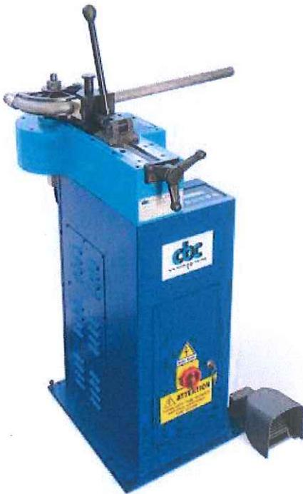
Digital, three-phase, and electric pipe bender to bend pipes of small and medium diameter of whatever type. Ideal to satisfy the exigencies in the plumbing, nautical, hydraulic, industrial and installation sectors.
