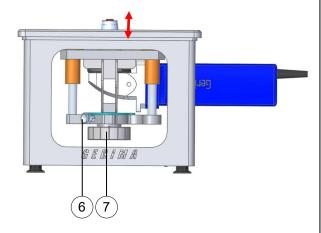
Once the bevel length has been set, a bevel should be milled on a test sample to check whether further height adjustments are required. These may be necessary.
