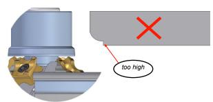
Milling head set to high (radius cuts into material).
