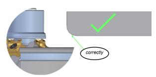
Milling head set correctly (radius fully formed with smooth transition to workpiece surfaces.)
