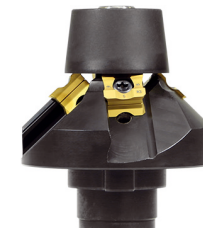
fig. 45°-radius-milling head with 4 cutting edges and guide roller, equipped with 4 mm-radius-indexable inserts of type R-K
