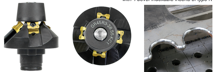
fig. 45°-radius-milling head with 4 cutting edges and guide roller, equipped with 4 x 3 mm-radius-indexable inserts of type R-K
