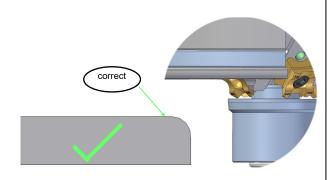
Guiding plate set correctly (radius fully formed with smooth transition to work-piece surfaces)
