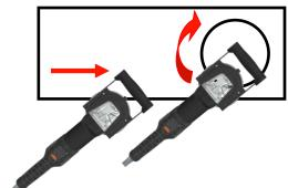
The arrows on the guide plate represent the direction of rotation of the milling head at the machining point.
