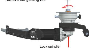
B Loosen the clamping screws with the Torx wrench T15 and replace the carbide inserts. The inserts must be fastened to the mounting seat on the milling head bymeans of the original locking screws (max. tightening torque: 4.0 –5.0 Nm).
