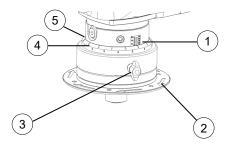
Once the bevel height has been set, a bevel should be milled on a test sample to check whether further height adjustments are required. These may be necessary because the precision of the scale is approximately ± 1 mm, depending on the type of milling head fitted.
