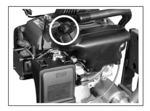
• If the motor is cold, position cold start indicator to 1 o 1.
