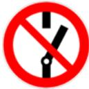
Before serving the machine always disconnect the machine from the power supply by removing the power cable from the socket !
