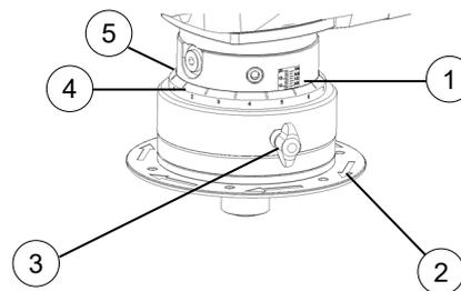
Once the bevel height has been set, a bevel should be milled on a test sample to check whether further height adjustments are required. These may be necessary because the precision of the scale is approximately  $\pm 1$  mm, depending on the type of milling head fitted.
