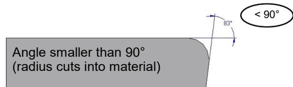
Angle smaller than 90° (radius cuts into material)
